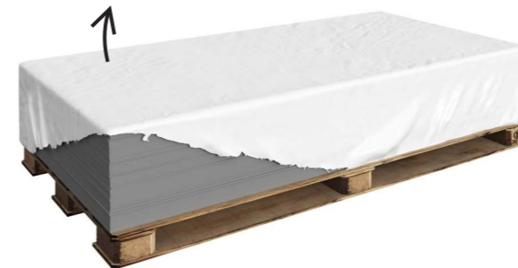
If the pallets are stored outside when they arrive at the building site, the plastic cover should be removed. The facade boards should be stored on the pallet or sleepers with max 500 mm distances.
