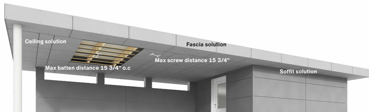
Screw and batten distances
