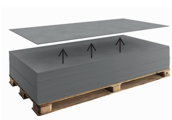
Do not drag products from the pallet, as it may leave permanent scratch marks. Lift the product by its narrow edge as it may break if handled incorrectly.
