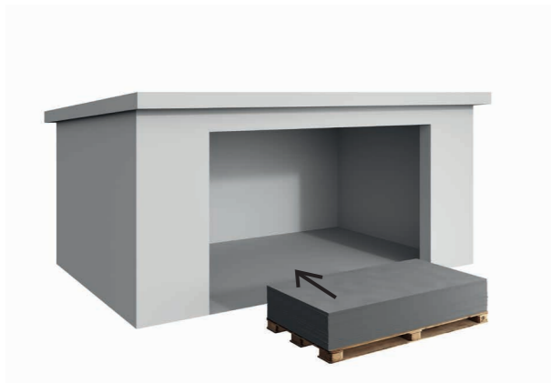
If storing on site for more than 2-3 weeks, the products should be kept under a roof. A maximum of 8 planks pallets can be stored on top of each other.
