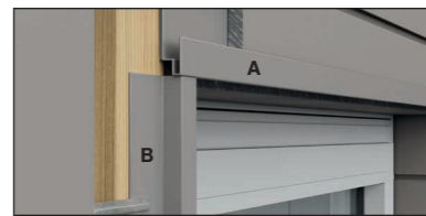
Picture 5 A. Swisspearl Plank Connect Window Profile B. Swisspearl Plank Connect External Corner Profile Small
