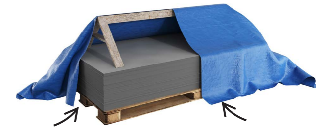
Replace the plastic with a tarpaulin. It is very important that there is ventilation all around the tarpaulin and also on top of the pallet under the tarpaulin. This is done to make sure that condensation is reduced as much as possible.
